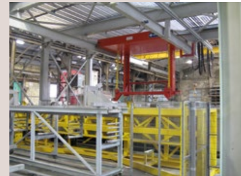
John Cockerill offers not only in-house tank construction and an extensive range of ventilation solutions, but also customized robotic systems that can be single or double column, as well as without column or inclination, and come with suction hood.
