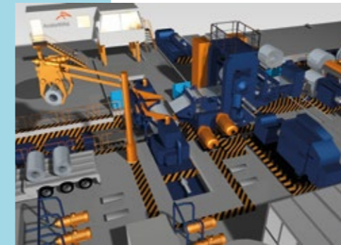
Stand-alone temper mill for automotive applications at ArcelorMittal Dofasco
