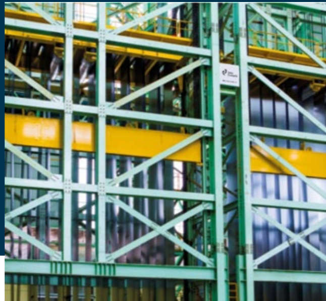
Double accumulator on Combi CAL-CGL, for automotive quality strip, VAMA, China
