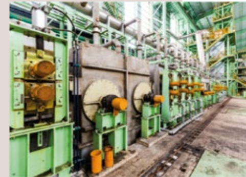
John Cockerill's multi-stage cleaning process is the centerpiece of its Electrolytic Cleaning Lines (ECL) and an essential component of number of other processing lines. The modular combination of spray, mechanical, chemical and electrolytic treatment steps is providing tremendous design flexibility and is ensuring excellent cleaning efficiency of all types of steel strip surfaces.
