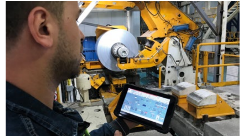
John Cockerill's "Virtual Operator Pulpit" allows for easy access to the line data, and all necessary process information, as well as to accept and implement the operators' control instructions.
