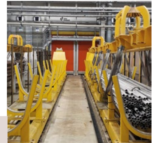
The fully automated Stainless Steel Tube Pickling Line supplied by John Cockerill to Sandviken, Sweden.
