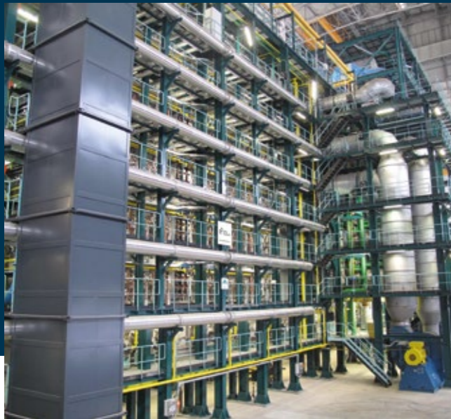
All radiant tubes vertical furnace with convective pre-heating chamber
