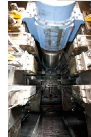
Stand-alone temper mill for automotive applications at ArcelorMittal Dofasco
