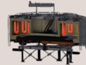
Rotary Hearth Furnace
